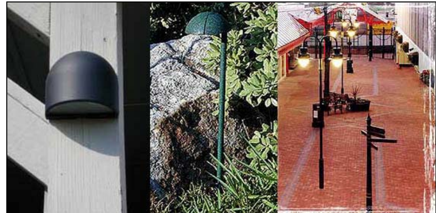
Figure 10 [examples of different levels of lighting to support the hierarchal structure system of the public spaces, to the left is bigger level post, in the middle is the medium and to the left is a small wall mounted lighting fixture]
